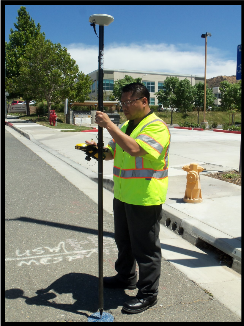
Raymond Chan, Engineering Technician II, using the Trimble Unit to collect coordinates of a pipeline for the Geographic Information System (GIS).
