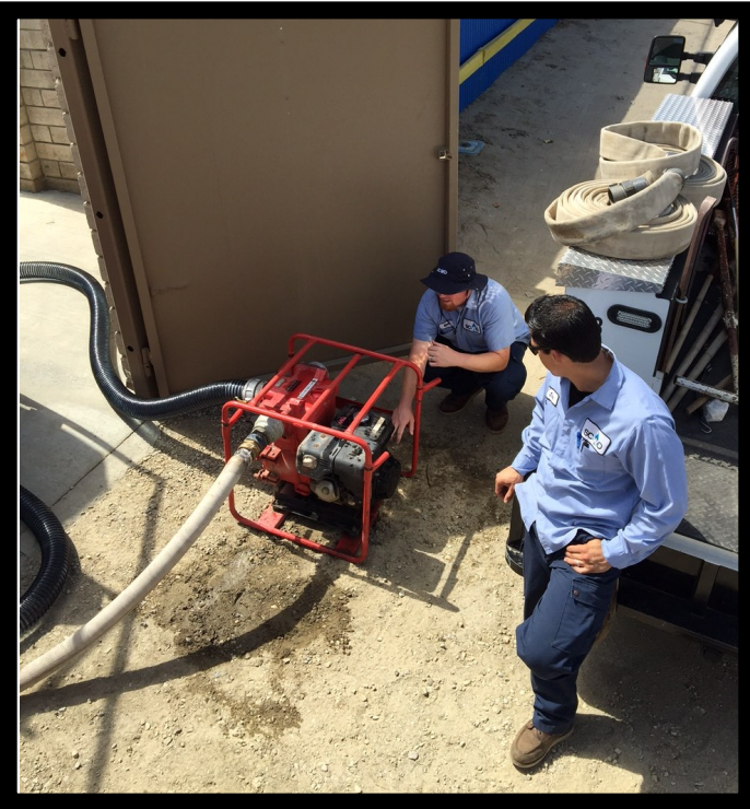
Ryan Bye, Senior Production Operator, and Jose Martinez, Production Operator I, are shown pumping non-potable water from a tank during maintenance, which helps reduce water waste.
