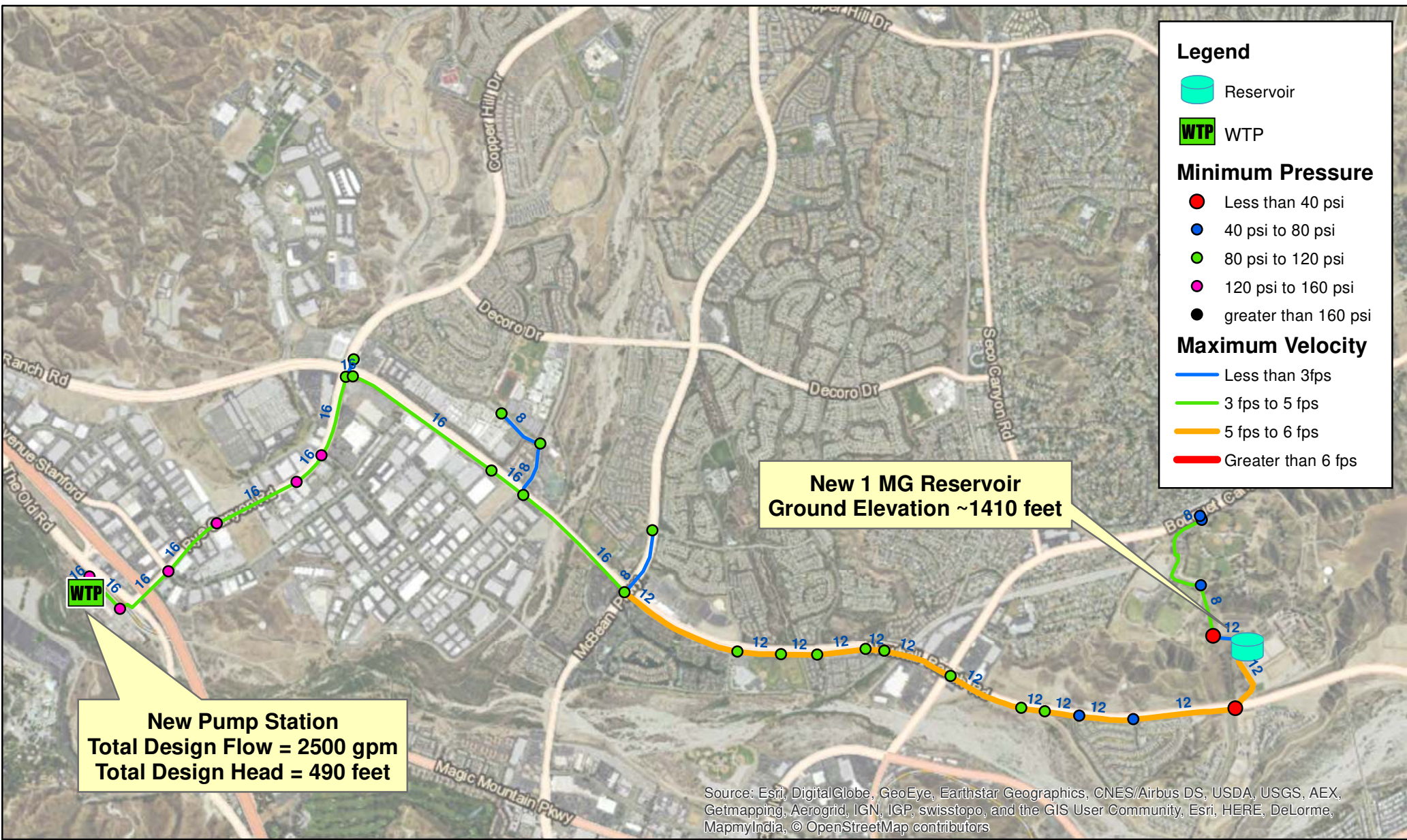
Figure 8 Minimum Pressures and Maximum Velocity Maximum Day Demands Phase 2A-1 with a Tank Alternative Recycled Water System Master Plan Castaic Lake Water Agency
